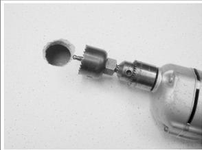
**1.** Using a hole saw, drill a 1½" hole in ceiling tile.
